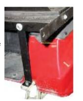
4. Install the step plate on the "L" bracket and leave the bolts loose for now.
