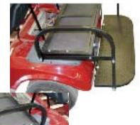
6. Install the new top struts. One set is for pre- $2000\frac{1}{2}$  and one set is for  $2000\frac{1}{2}$  to present.
