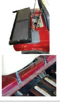
**3.** Install the "L" bracket to the inside frame and attach to the rear bumper mount. Leave the bolts loose for now.
